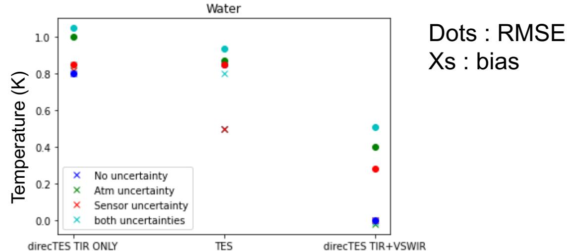
Significant bias for direcTES (TIR only) and TES which makes most of the RMSE
